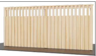
1.8m High timber board and batten fence (0.3m permeable top). Battens to face the street/JOAL*
