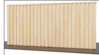
1.8m High timber board and batten fence with capping. Battens to face the street/JOAL*
