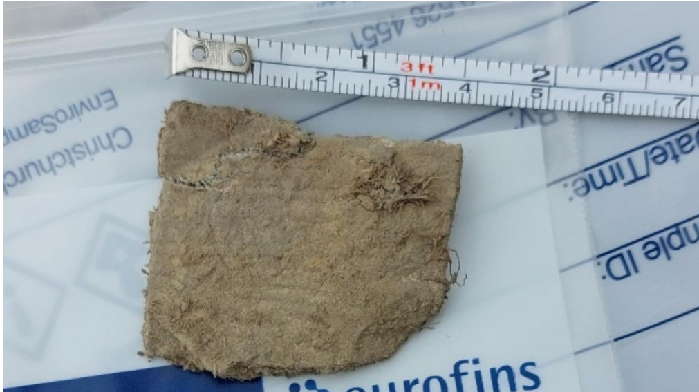
Photograph B9: ACM fragment identified in surficial soil (approximately 0.15 m bgl) at 6HA2. Fragment removed from site.
