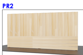
1.8m High timber paling fence combined with retaining (base to be adjusted to suit site levels, 0.5m max)
