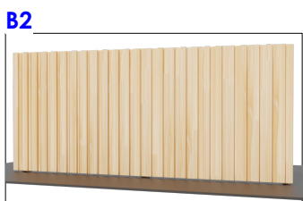
1.8m High timber board and batten fence. Battens to face the street/JOAL
