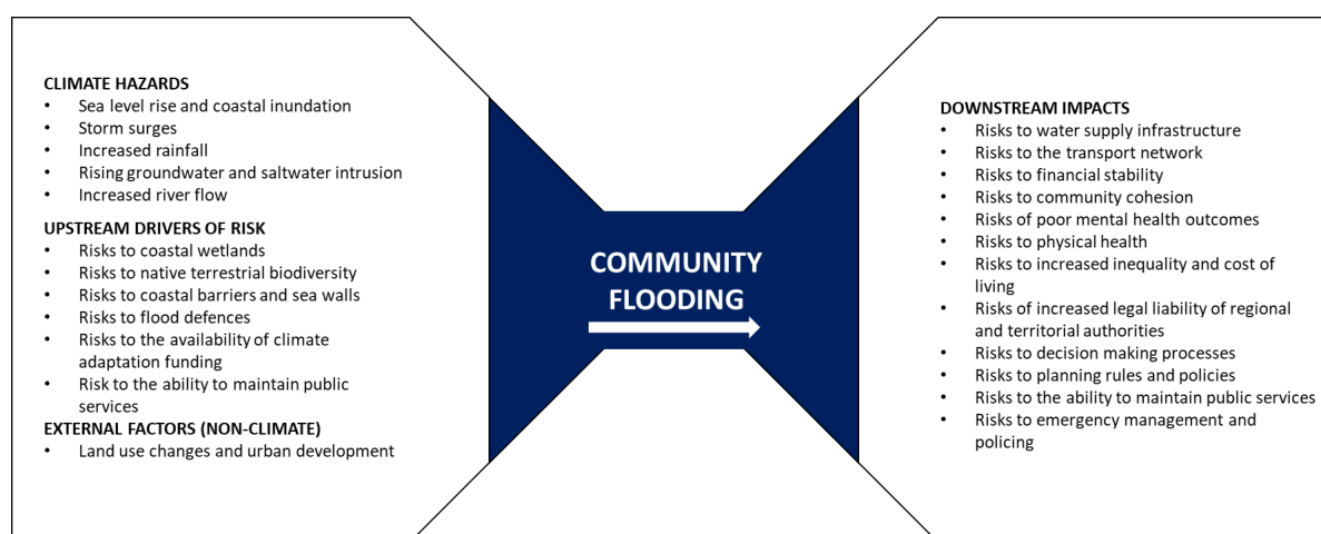
Figure 20.5: Bow tie diagram showing upstream hazards, drivers and external factors which lead to community flooding risk, and the downstream impacts of this risk.
