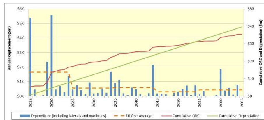
Figure 6-1: 50 Year Sewer Mains ORC Profile
